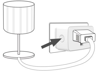
2. The LED on socket switch will flash three times to indicate all memory are cleared.
