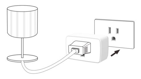
2. Press 'Pair Button' once (LED will start to flash), with the remote control press the **'ON'** button intend to be paired; LED on socket switch will quick flash 5 times to confirm that the remote control is now paired.
