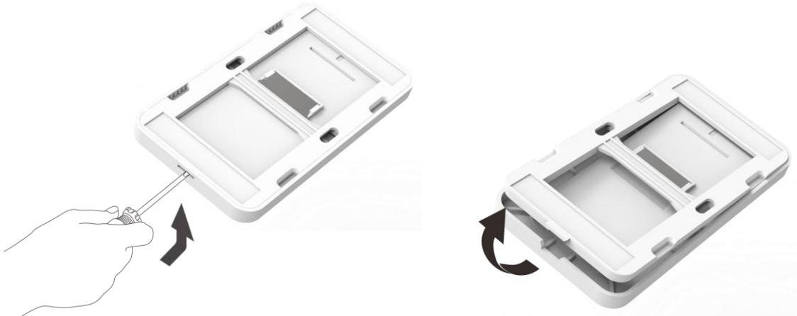
2. Position the back magnetic holder onto surface making sure the arrow is facing up then affix tightly with 2 screws.
