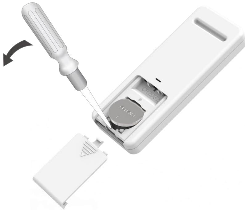
3. Insert new 3V CR2032 battery making sure the positive symbol is facing upwards and slide back the battery cover.
