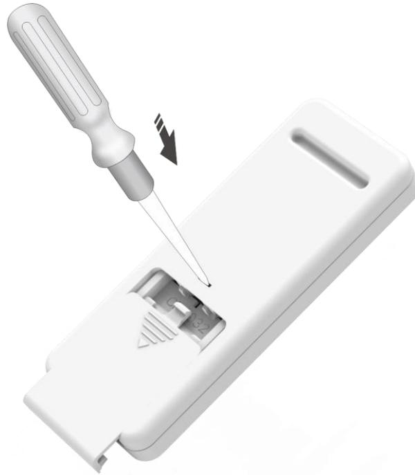
2. Insert flat headed screwdriver and slightly lift up to remove battery.
