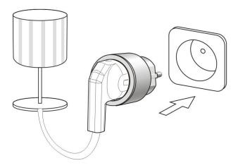
3. Within 6 seconds press **ON** button once to pair, LED will flash and load will flash twice to confirm that pairing is successful.
