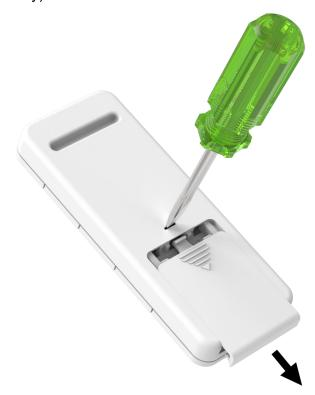
2. Insert flat headed screwdriver and slightly lift up to remove battery.
