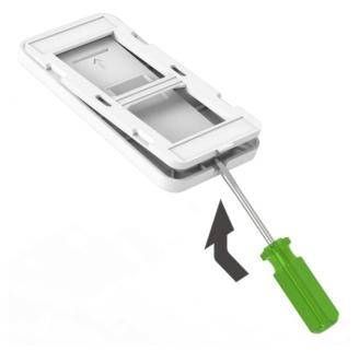
2. Position the back magnetic holder onto surface making sure the arrow is facing up then affix tightly with 2 screws.
