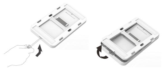
2. Position the back magnetic holder onto surface making sure the arrow is facing up then affix tightly with 2 screws.
