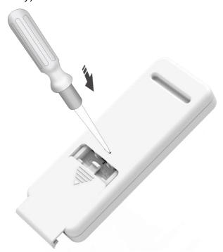
2. Insert flat headed screwdriver and slightly lift up to remove battery.
