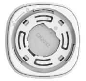
3. To close the battery cover, align the arrow at the unlock position and turn clockwise to tighten the battery cover.
