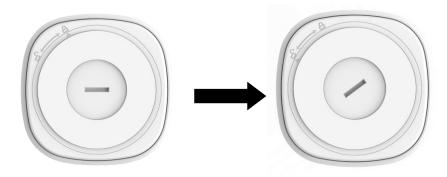
2. To change battery, insert new 3V CR2032 battery making sure the positive symbol is facing upwards.
