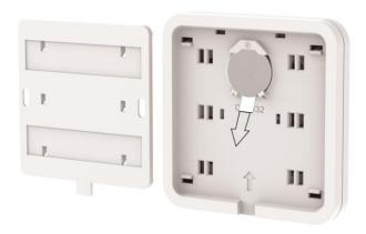
4. Or replace with a new 3V CR2032 battery making sure the positive symbol is facing upwards.
